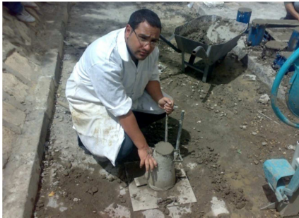
Figure 10. Slump test.
