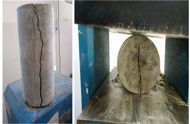
Figure 14. Test of cylinder.
