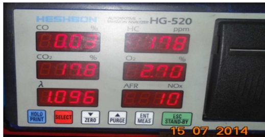
Figure 10. Exhaust gas composition after rinsing injector with new equipment and new solution
