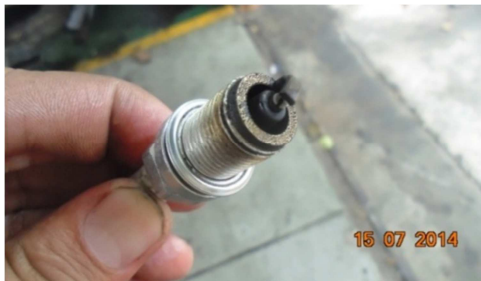
Figure 11. Soot on top of the spark plug after rinsing injector
