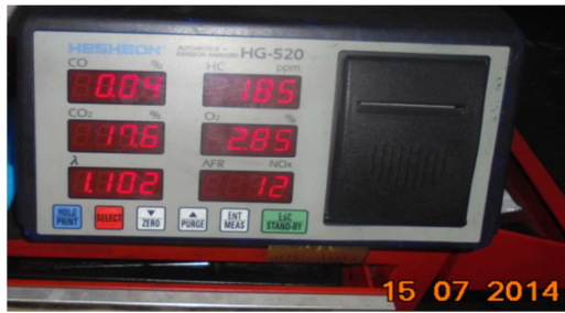
Figure 9. Exhaust gas composition before rinsing injector
