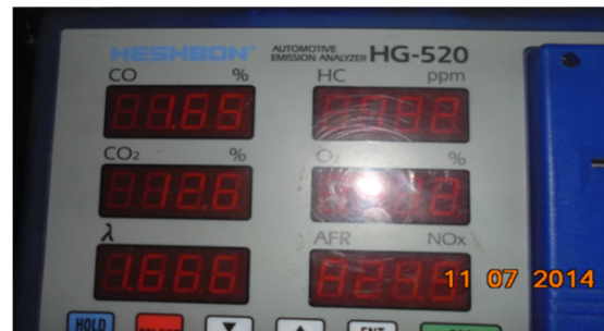
Figure 13. Exhaust gas composition after rinsing injector with Fuel Injection solution
