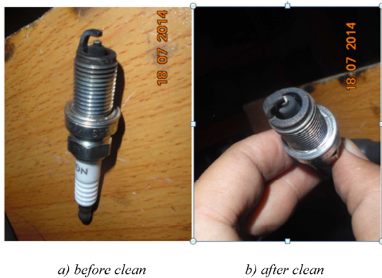
Figure 15. Soot on the spark plug before and after cleaning by new equipment and new Solution
