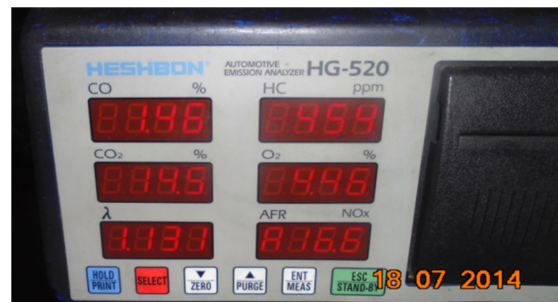
Figure 14. Exhaust gas composition after rinsing injector with new solution
